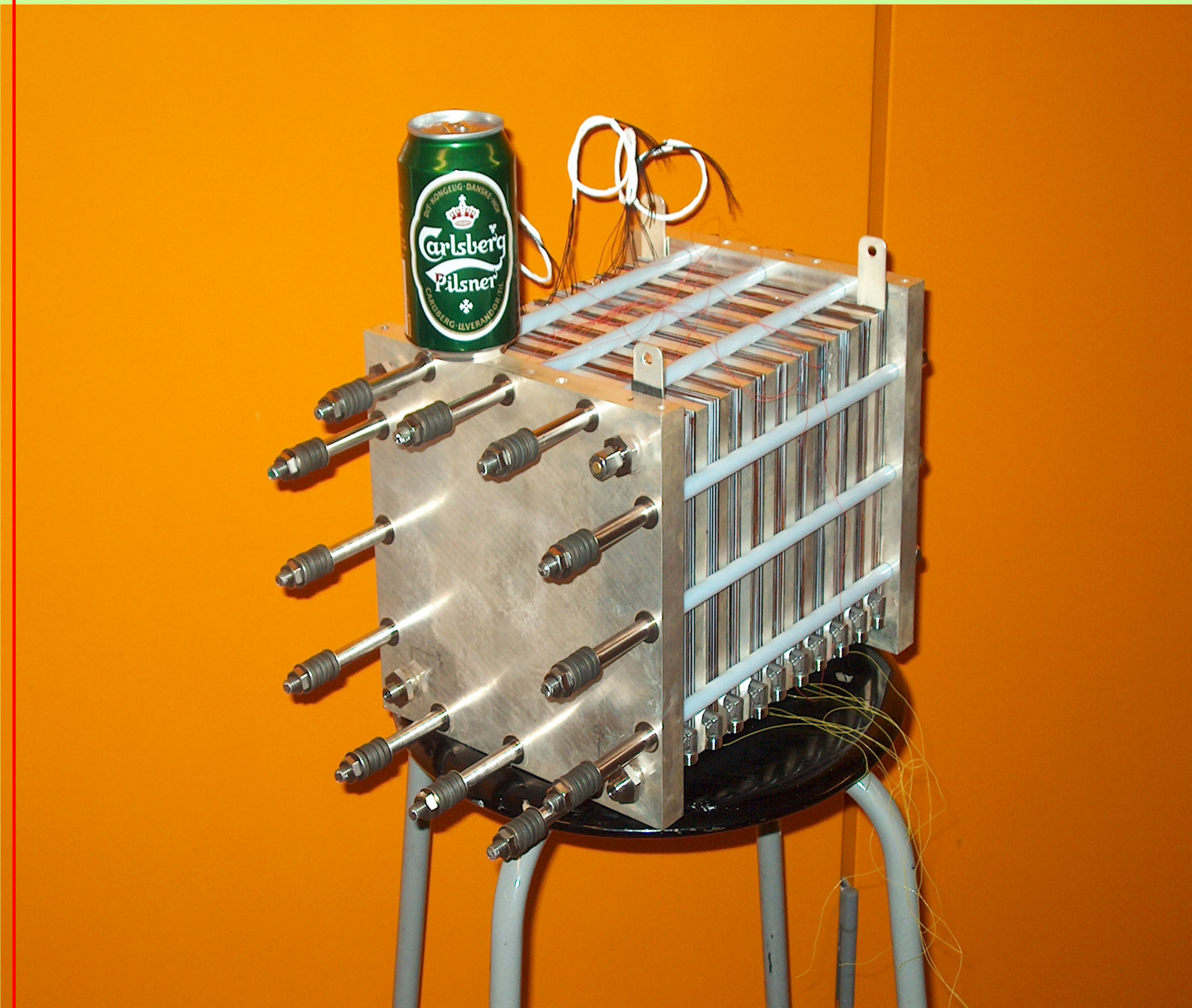
1 kW high temperature PEMFC stack, consisting of 40 cell stack with electrode area of 256 cm 2 . Constructed in the AMFC project (EUF5)
