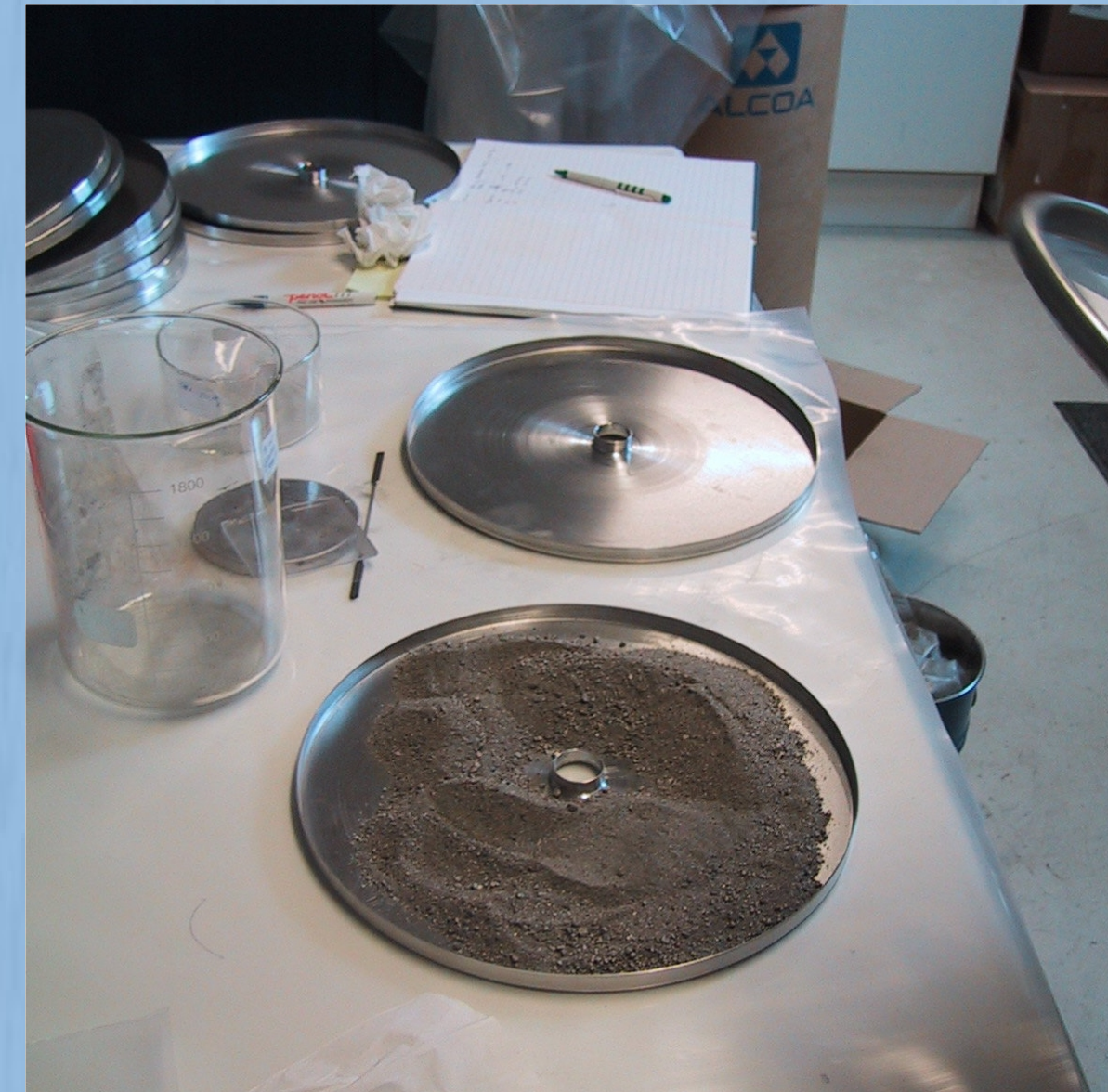
Left: Cross section of final tank. Mid: The final tank. Volume 17.5 L. 29 kg hydride. Right: one compartment during filling (in air)
